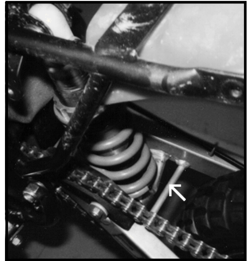
Fig. 2. Make sure that when the shock is fully collapsed that the spring or retainer does not make contact with the cross bar (arrow).
