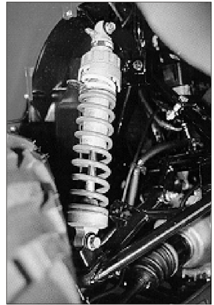
Fig. 1. Front shock installation. Note that the shock body is at the top with the shaft pointing down. ARS shown is in the unloaded position.
