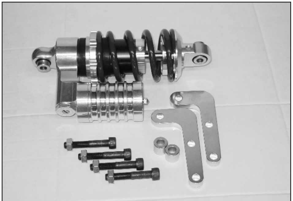
Fig. 1: Mounting hardware includes four bolts and nuts, two mounting plates, two spacers and a flat washer (not shown). The shock is equipped with a spring rate that supplements the stock spring rate. The stock spring carrier complete with linkage must remain in use with this shock.
