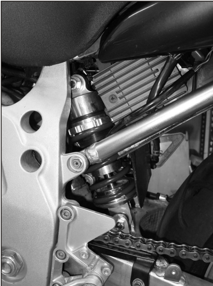
Fig. 5: Shock installation complete as seen from the left side of the motorcycle. After the initial ride, check all the bolts and nuts for proper torque. Refer to the information in this guide and the set-up information on adjustable shocks in guide # UAADJ.
