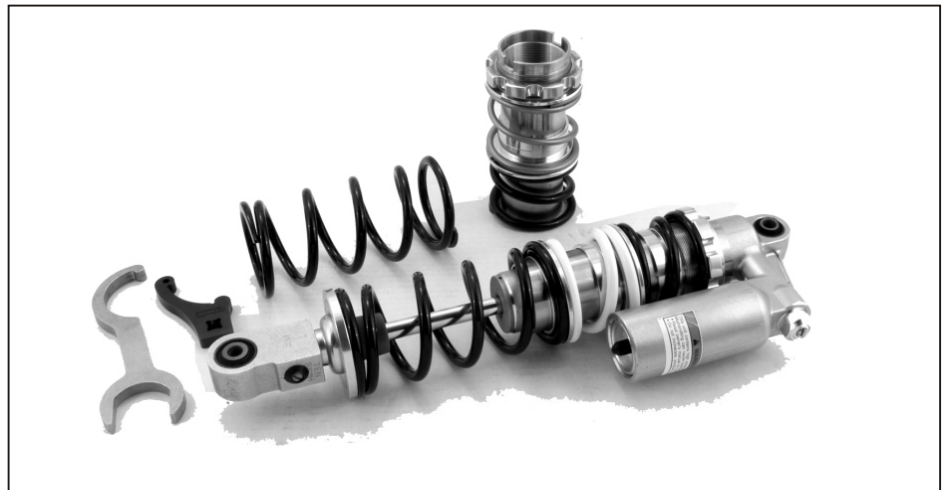
Fig. 1-- Works triple-rate springs kits with sleeves are designed for cast aluminum OEM shocks. The sleeves provide a surface for the springs and separators to slide on. Each kit is specific to your weight, riding type and arm configuration. They are available in motocross, cross-country, stadium and recreation configurations.
