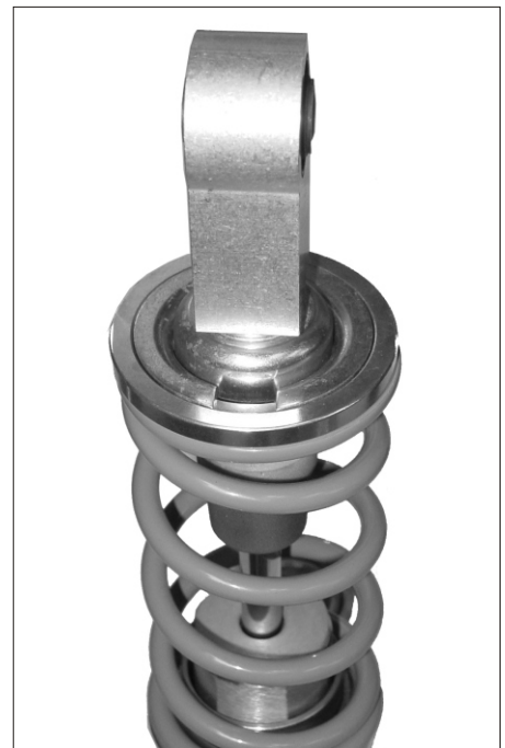
Fig. 9--Install the retainer between the stock bumper cup and the adaptor ring.
