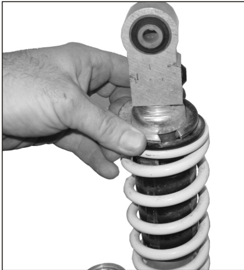
Fig. 4-- Remove the retainer. With the preload backed off the stock spring, it should be possible to remove the retainer by hand.
