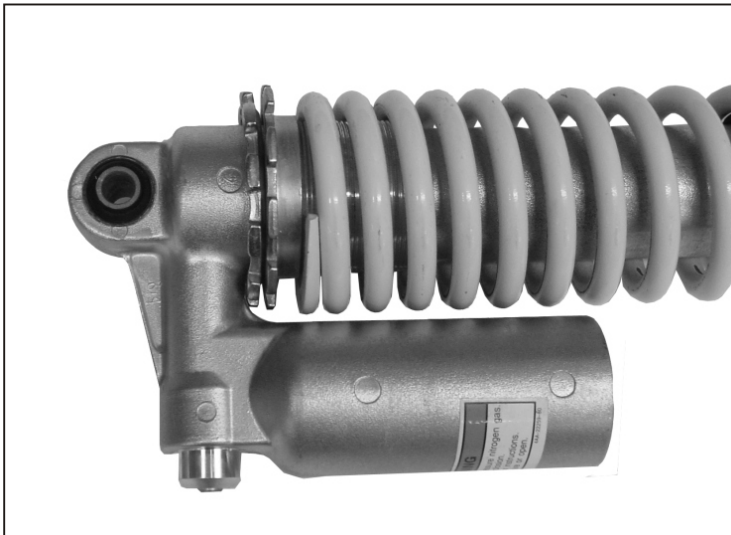
Fig. 4-- Remove the retainer. With the preload backed off the stock spring, it should be possible to remove the retainer by hand.
