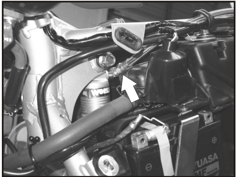
Fig. 1. Arrow indicates position of hose as it angles toward the airbox. The hose then arcs over the top of the air box along side the wiring loom.
